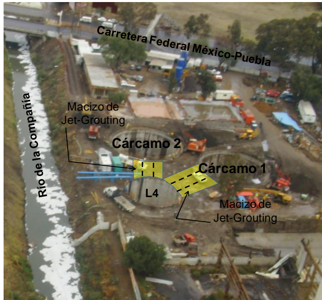
Figure 2. Distribution of the pumping plant
