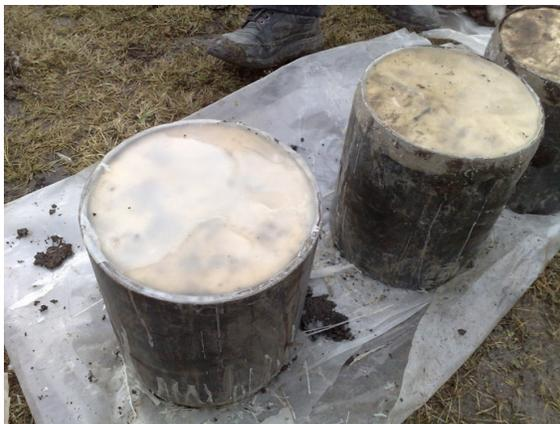
Figure 2. Waxed peat samples inside the samplers
