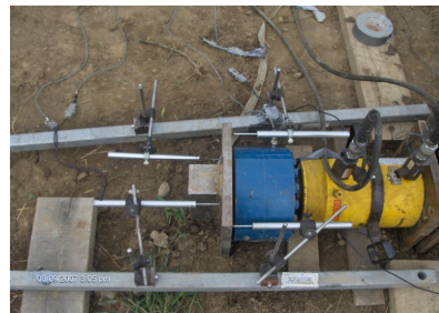
Figure.12.b. Lateral loading setup zoom-in for the hydraulic jack-load cell and the four LDTs setup.
