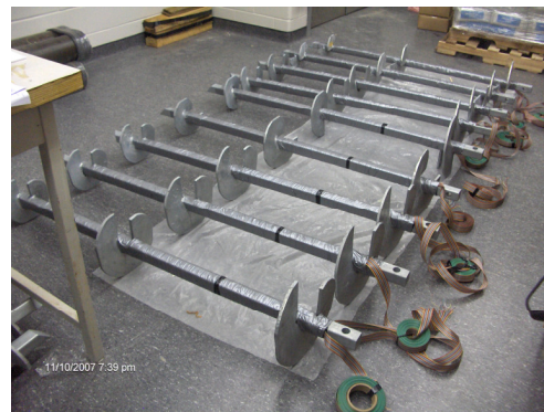
Figure 4.b. Finished instrumented lead sections
