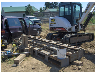
Figure.12.a. Lateral loading setup
