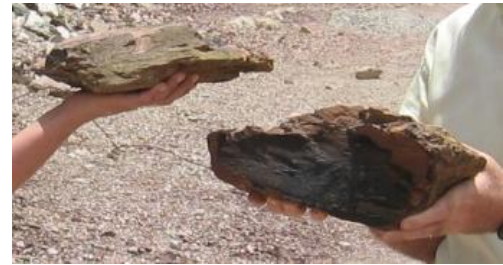
Figure 3. Phyllite schist samples collected for direct shear tests
