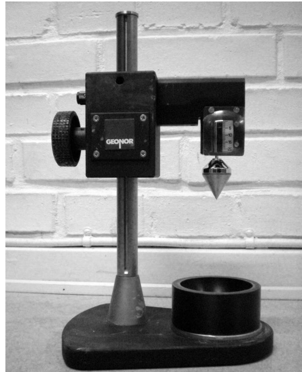
Figure 3. The Fall Cone Apparatus used for the tests.
