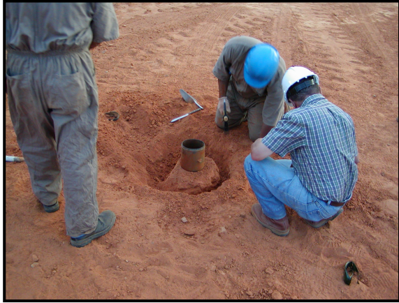
Figure 5. Undisturbed samples with ring.
