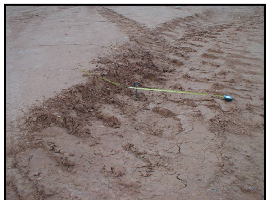
Figure 17. Evidence left by the step of a truck wheel on area in court of collapsible material after rain
