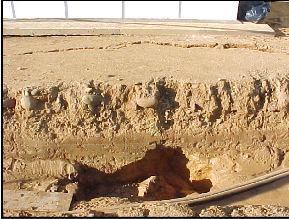
Figure 13. In-situ measurement of the induced settlement in collapsible soils of area of Jose.
