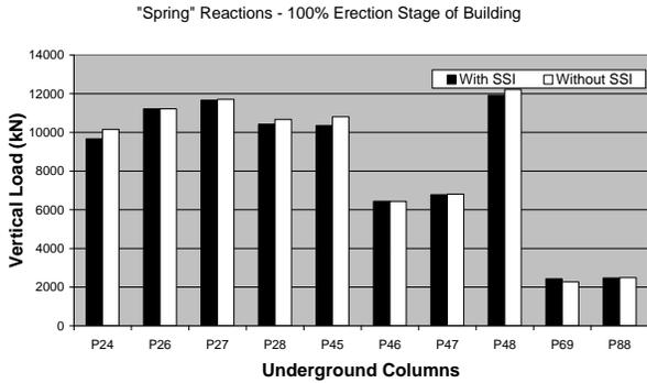
Figure 9. Vertical column loads with and without SSI
