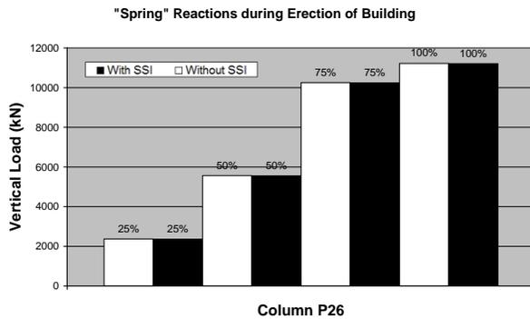
Figure 10. Vertical load of column 26 at distinct stages
