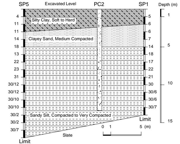
Figure 2. Typical geotechnical profile of the site
