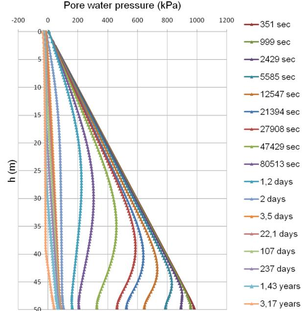
Figure 8: Evolution of the pore water pressure along the VCL of the initially saturated backfilled slope (Case 3)
