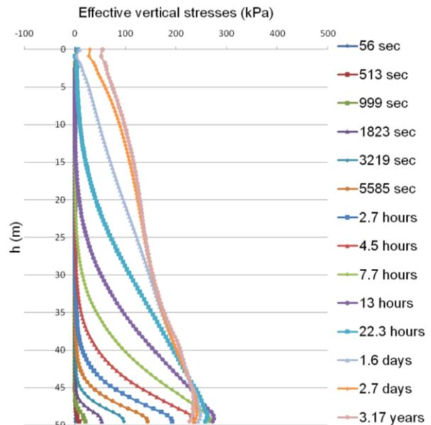
Figure 9: Evolution of the effective vertical stress  $\sigma'_v$  along the VCL within the backfilled slope (Case 3)
