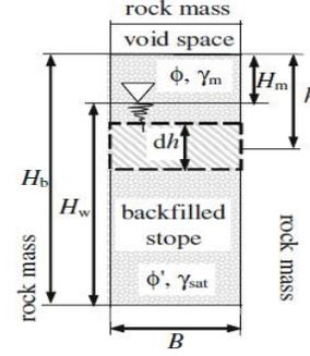
Figure 1: A vertical stope with partially submerged backfill (adapted from Li and Aubertin, 2009a)
