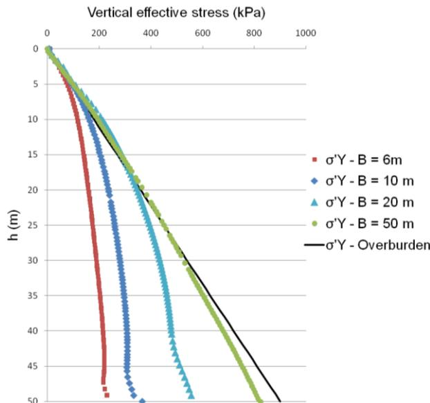
Figure 5: The effect of stope width B on the vertical stress along the VCL (Case 1).
