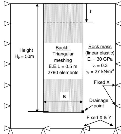
Figure 2: Stope geometry and finite element mesh
