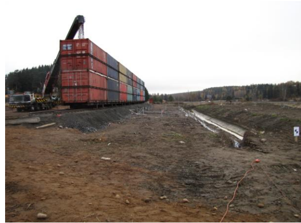
Figure 6. Test site and loading of the containers on the second loading day.
