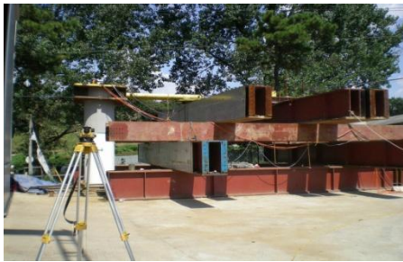
Picture 1. Lateral Load Test
