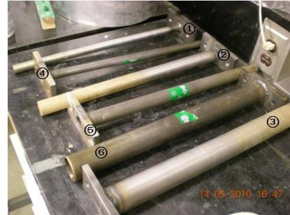
Figure 3b. Model piles and thin-wall tubes.
