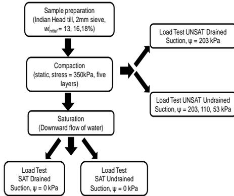
Figure 5. Flow chart of the testing program.
