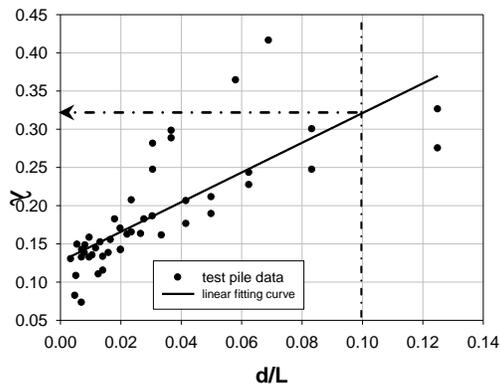
Figure 13. Relationship between the variation of  $\lambda$  coefficient and the ratio between pile diameter,  $d$  to pile penetration,  $L$  using the data from Vijayvergiya and Fotch, (1972).
