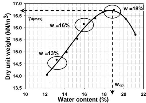
Figure 2. Compaction curve for the Indian Head till.
