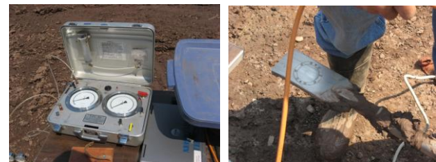
Figure 3 Dilatometer control panel (left) and blade (right)
