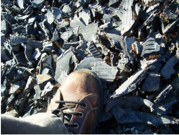
Figure 2. Tire Derived Aggregate (photo by D. Staseff)
