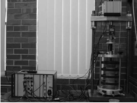
Figure 2 : The triaxial apparatus.
