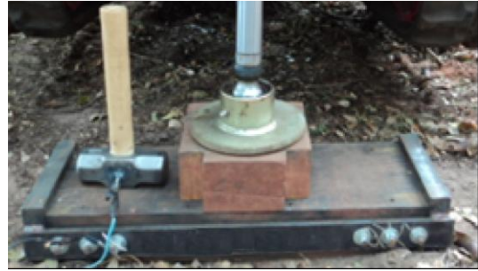
Figure 7. Smaller shear beam placed in the rear of the pushing equipment.
