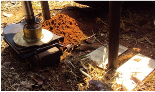
Figure 9. Seismic source placed at the front of the pushing equipment.
