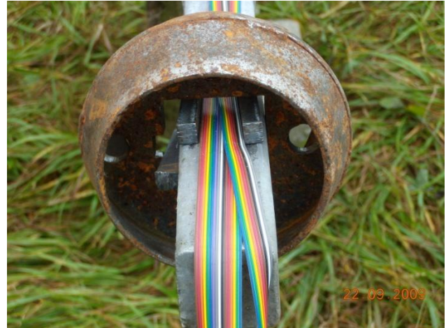
Figure 2. Displacement disk attached to an extension.
