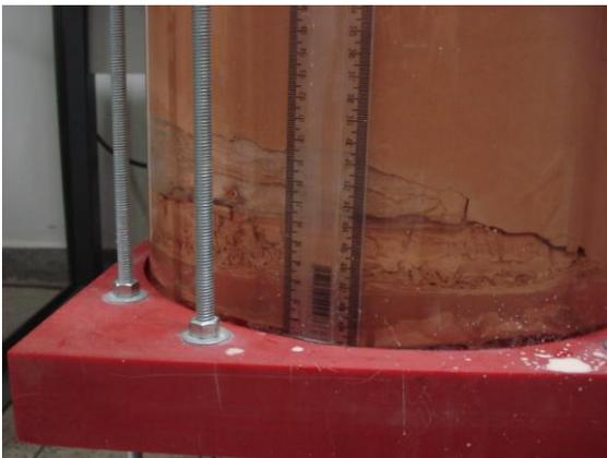
Figure 9. Shrinkage at the bottom of model after reversal of polarity
