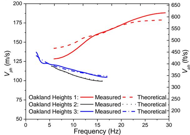
Figure 10. Dispersion curves at Oakland Heights landfill
