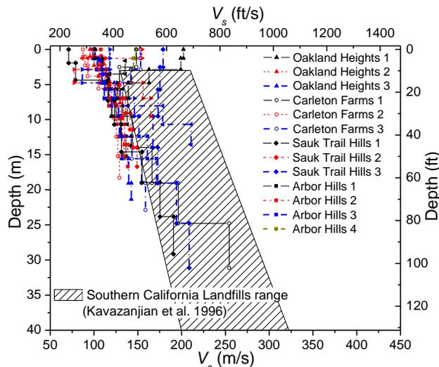
Figure 17.  $V_s$  profiles from this study and literature
