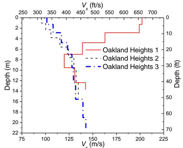
Figure 11.  $V_s$  profiles at Oakland Heights landfill
