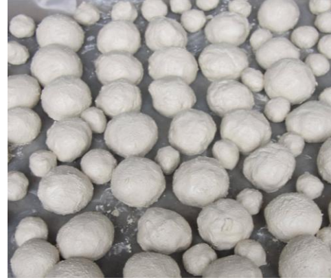
Figure 6. Clay balls made for simulating lumpy soil
