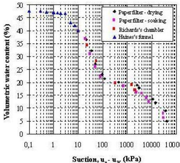
Figure 5. Soil water characteristic curve – area 2, Lafayette (2006).
