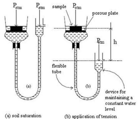
Figure 3. Illustration of Haines funnels equipment.
