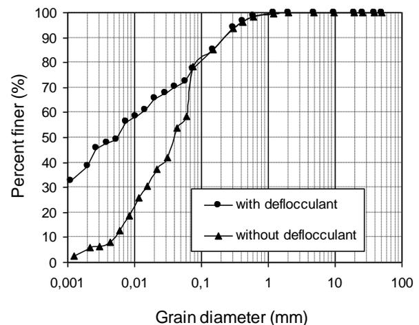
Figure 1. Granulometric test results – area 1.
