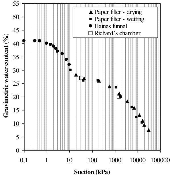
Figure 4. Soil-water characteristic curve research area 1 - Silva & Coutinho (2007).
