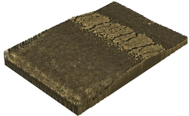
(b). Overtopping and formation of rills
