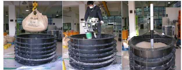
[1] Sand raining [2] 1 st Compaction [3] Pipe installation
