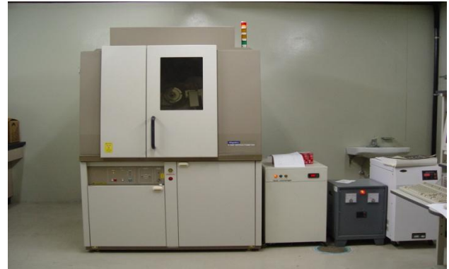
Figure 2. XRD principles and equipment
