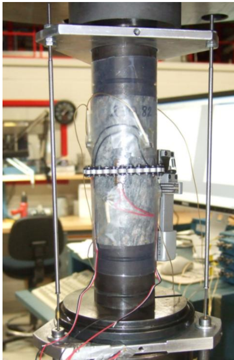
Figure 10. A Smaland granite specimen ready for testing, the specimen was monitored by AE sensors, vertical and horizontal strain gauges, LVDTs for axial deformation and extensometer for circumferential strain (Courtesy of ISRM Commission on Spalling Prediction). 4.1 Smaland granite
