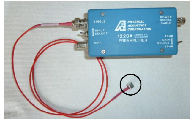
Figure 8. AE transducer (circle) and pre-amplifier used for AE monitoring.
