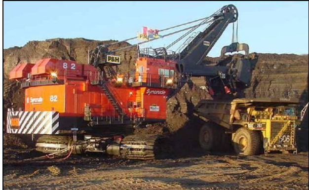
Figure 11 P&H 4100C Shovel Loading a 797B Hauler
