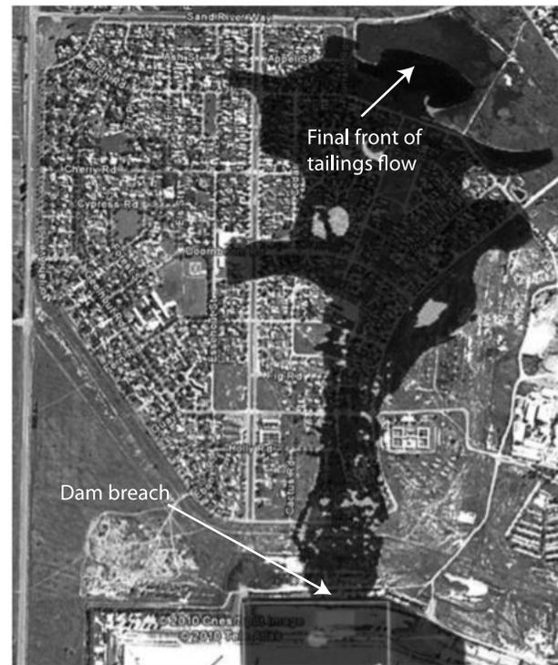
Figure 5. The result of Merriespruit tailings dam failure simulation superimposed on satellite imagery (Google Earth 2010)
