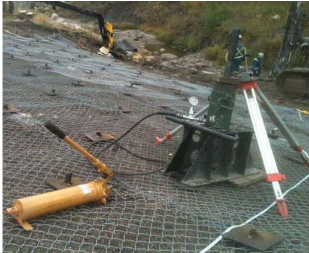
Figure 7. Soil nail pullout test setup
