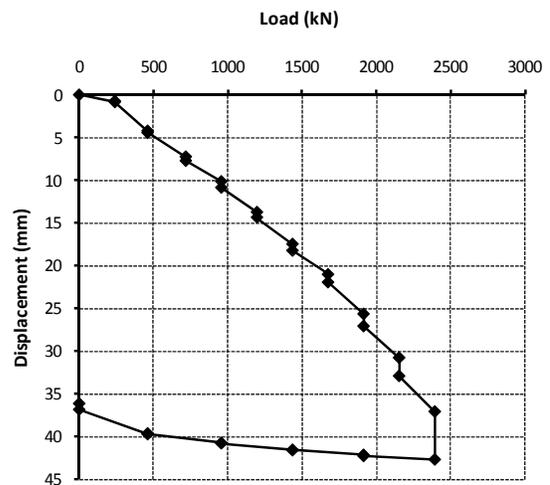
Figure 6 Load x settlement curve for piled raft with two piles
