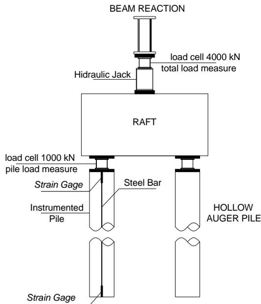
Figure 4. Instrumentation scheme
