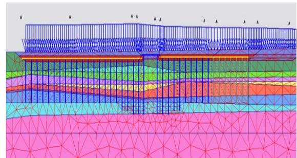
Figure 7. PLAXIS Model: Longitudinal Direction (Plate Elements)
