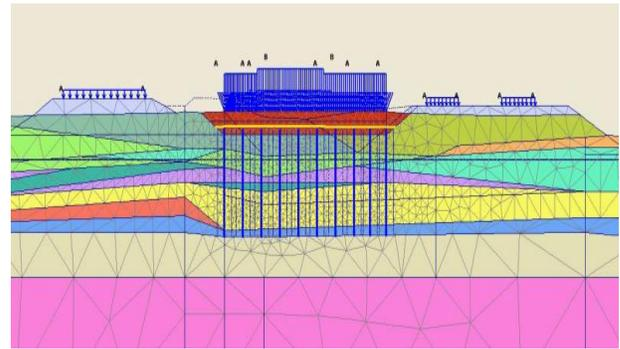
Figure 6. PLAXIS Model: Transverse Direction (Plate Elements)
