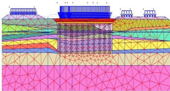
Figure 9. PLAXIS Model: Transverse Direction (Equivalent Soil Block)
