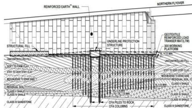
Figure 2. Surface profile and ground improvement
