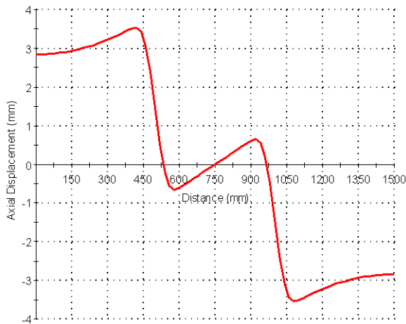
Figure 18. Distribution of axial displacement relative to the borehole.
