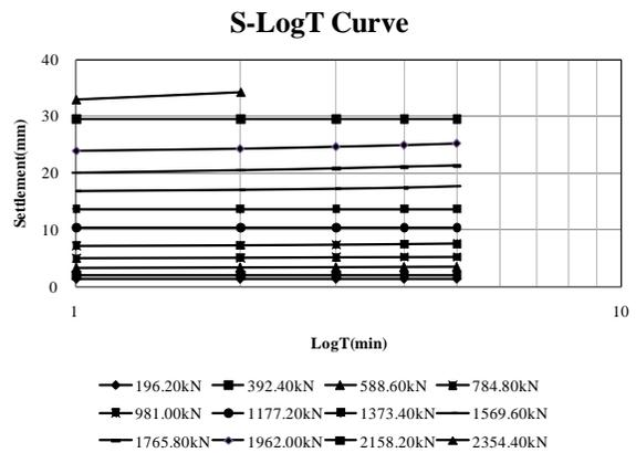
Figure 7. S-LogT curve of TP1 for each load step
