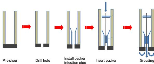
Figure 1. Pile tip grouting procedure
