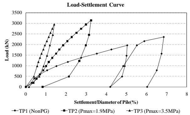
Figure 15. Load-settlement curves of test piles
