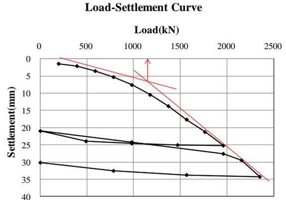
Figure 5. P-S curve of TP1
