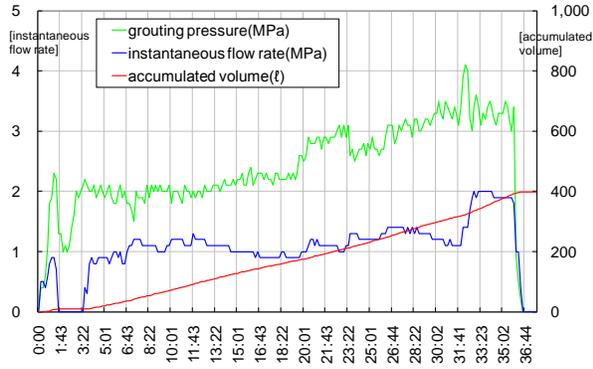
Figure 4. Grouting results for TP3
