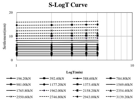
Figure 11. S-LogT curve of TP2 for each load step
