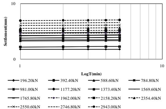
Figure 14. S-LogT curve of TP3 for each load step
