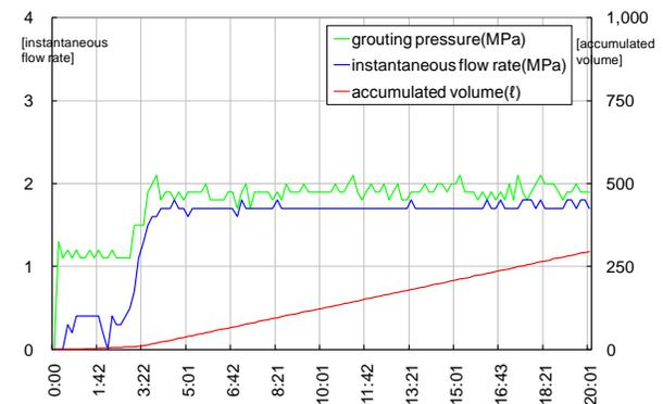
Figure 3. Grouting results for TP2
