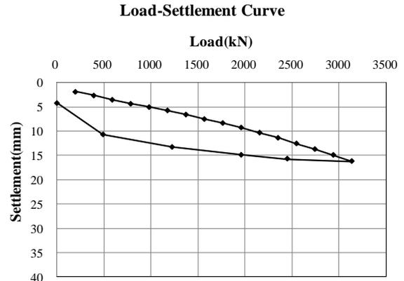
Figure 9. P-S curve of TP2
