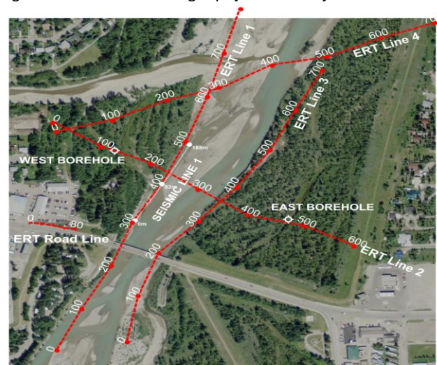
Figure 2 Locations of the geophysical survey lines
