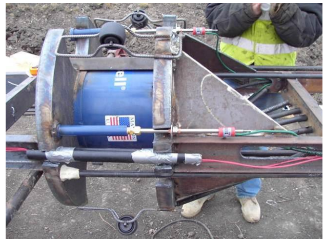
Photo 1. Osterberg Load Cell
