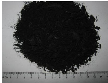
Figure 2. View of the tire buffings used in this study
