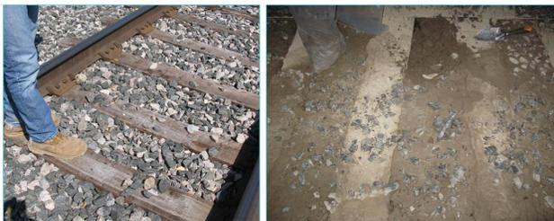
Figure 1. Exposure of clean ballast (left) and heavily fouled ballast (right), on the surface of the rail embankment.
