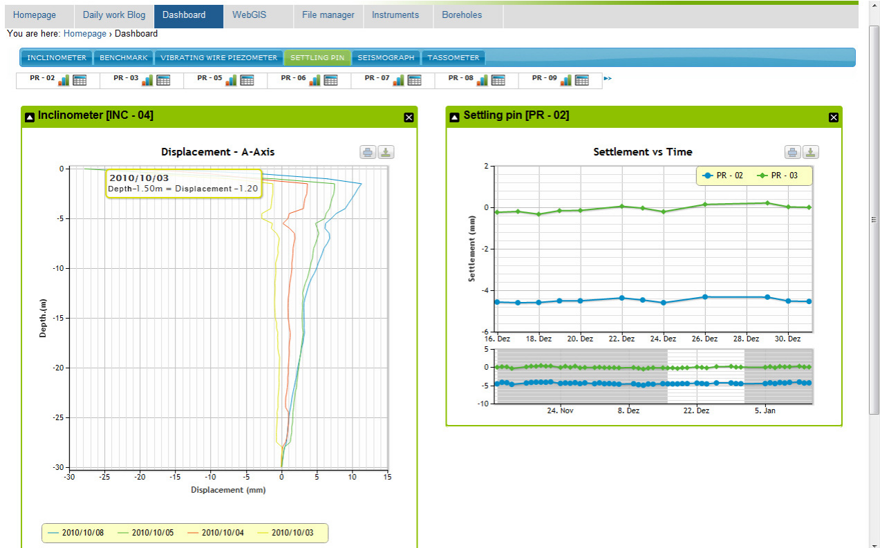
Figure 6. Dashboard of dynamic graphics showing data of geotechnical instrumentation (inclinometer at the left; and settling pin graph at the right).
