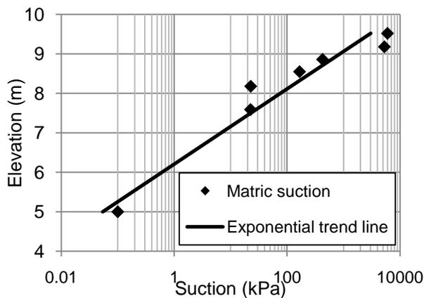
Figure 4. Initial condition of negative pore-water pressure
