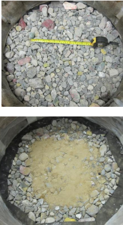
Figure 3. Photographs showing surface directly beneath the geomembrane prior to: a) test 1 and b) test 2.
