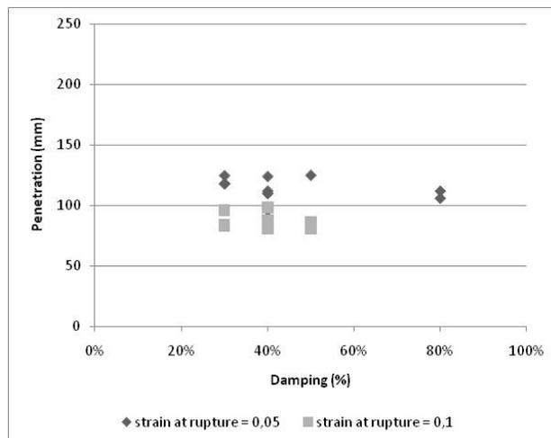
Figure 4. Variation of penetration with damping (models 19 to 40).
