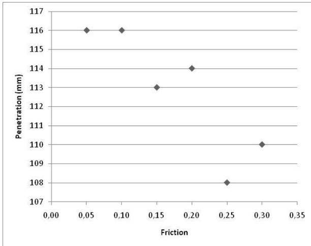
Figure 6. Variation of penetration with friction (models 45 to 50).
