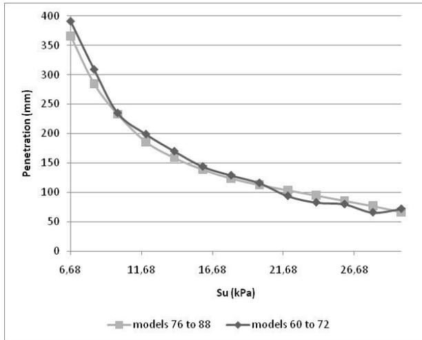
Figure 10. Variation of penetration with undrained strength (models 57 60 to 72 and 73 76 to 88).
