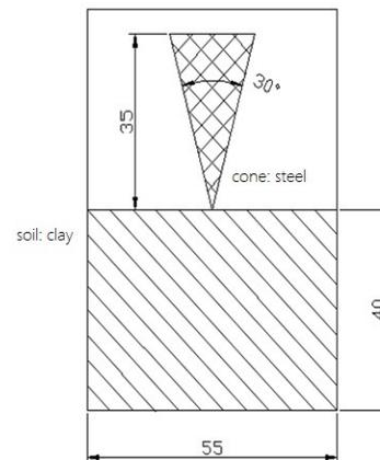
Figure 2. Numerical fall cone penetration test dimensions in cm.
