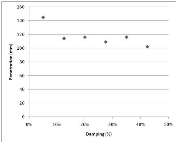
Figure 7. Variation of penetration with damping (models 51 to 56).
