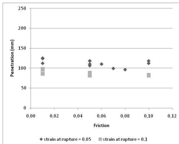
Figure 5. Variation of penetration with dynamic friction (models 19 to 40).
