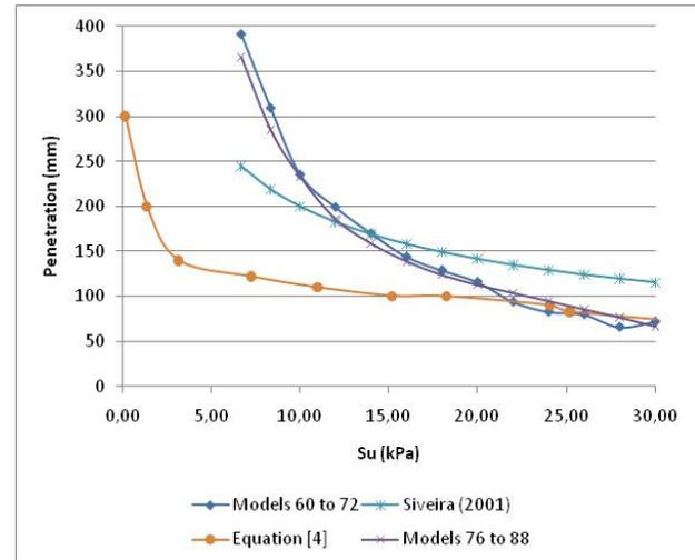
Figure 11. Comparison between the numerical models 57 to 88 and literature references.
