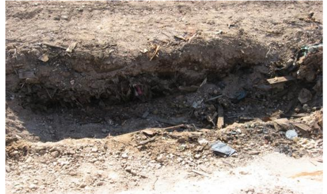
FIGURE 7 Test Pit showing MSW layer
