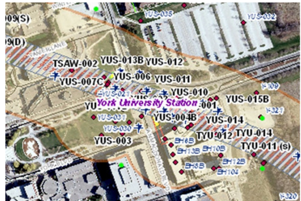
Figure 4: GECMS Spatial view of York University Station site borehole layout
