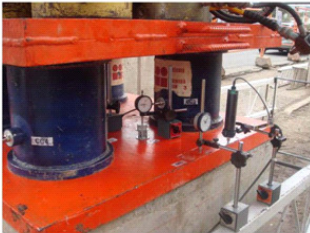
Figure 5. General view of head instrumentation for a compression test
