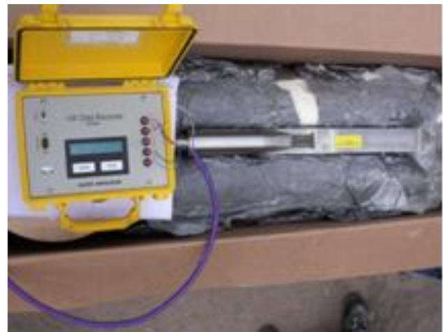
Figure 1. Piezo-cell and measurement box
