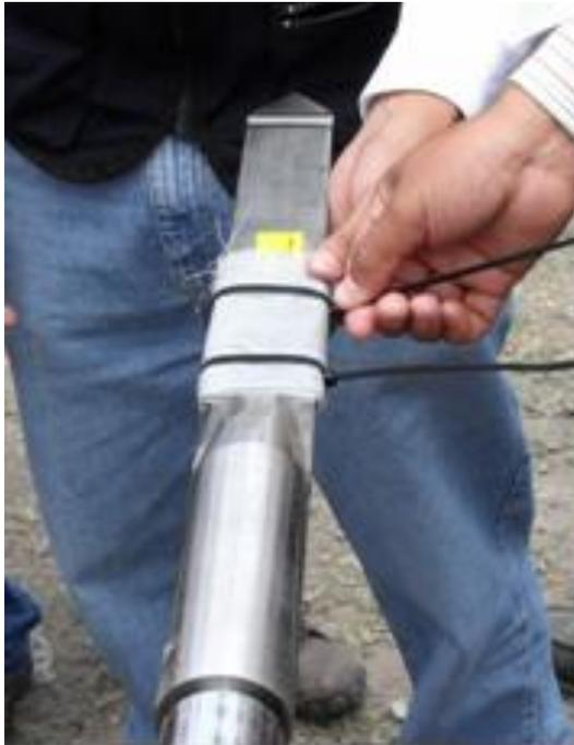
Figure 2. Protecting the piezometer of the piezo-cell
