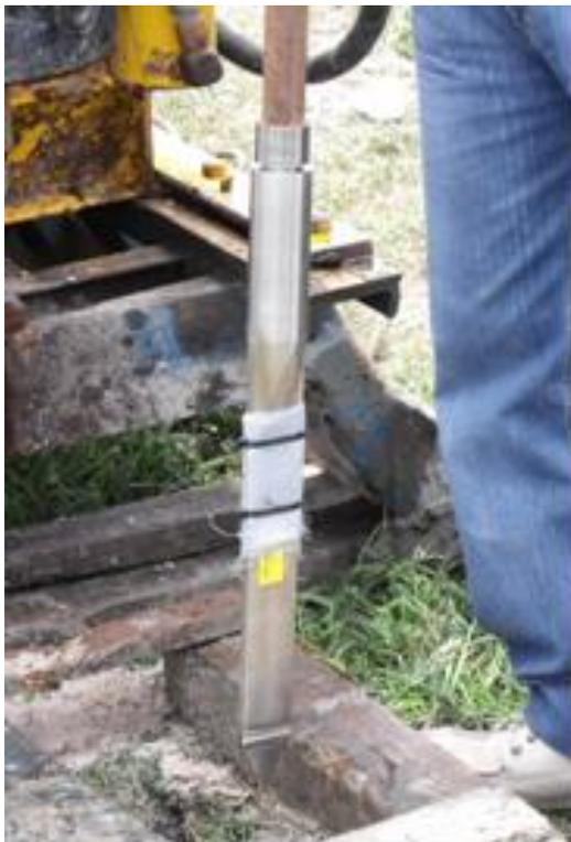
Figure 3. Piezo-cell ready to be driven
