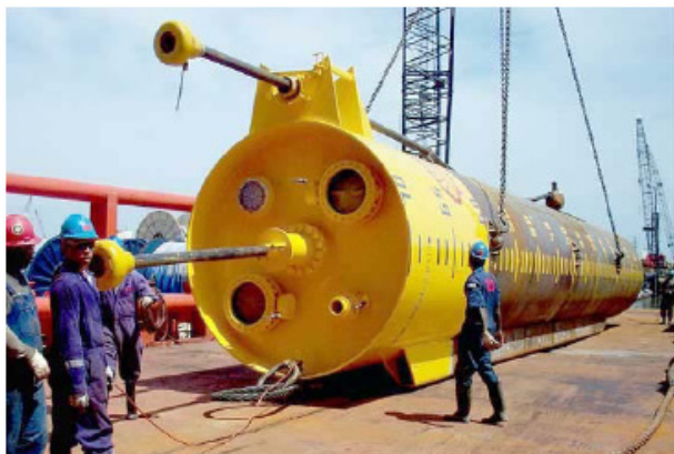
Figure11. Anchor / suction pile is shown.
