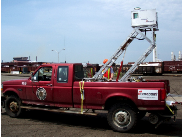
Figure 5. The TITAN system (silver box) is a multi-LiDAR scanner mounted on a rail-capable vehicle.
