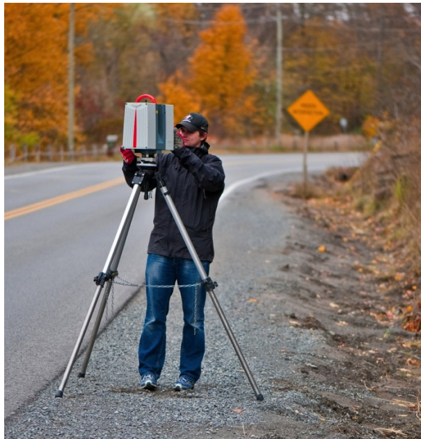
Figure 3. Field deployment of a static terrestrial LiDAR scanner (Leica HDS6000)
